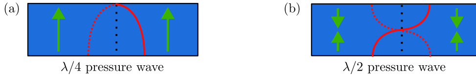
Figure 4.1: (a) Standing-pressure \lambda/4 -mode in a microfluidic channel with particles being pushed to the top of the channel (green arrow). (b) \lambda/2 -mode with particle focusing at the channel center.
