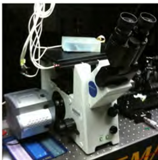
Figure A.3: Photo of the experimental setup described in Chapter 4 showing the microscope with CCD camera attached into its left side and the electrical connections for the chip going into a white, protective box placed on the top stage with optical access from below (inverted microscopy). Figure adapted from our paper [76].
