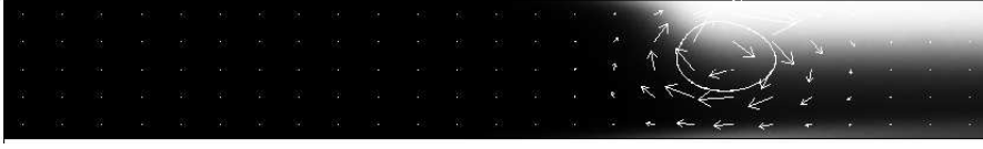
Figure 4.3: The flow roll set up in capturing of magnetic beads. The arrows show the difference between the fluid velocity and unperturbed Poiseuille flow setting up the indicated vortex. The grey scale indicates the concentration of beads. The initial concentration is 10^{13} \text{ m}^{-3} and the maximum flow speed is 100 \text{ } \mu\text{m/s} .
