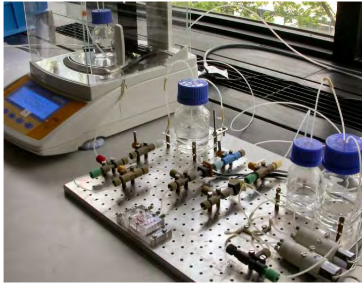
Figure B.3: Picture of the setup for measuring hydraulic resistance. The equivalent flow diagram is identical to that in Fig. 5.6 but without the switching valves (1-4). In this picture a chip holder similar to that in Fig. 8.7(b) is inserted between the pressure sensors.
