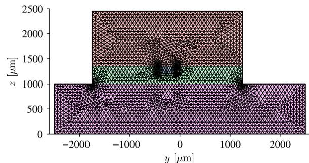
FIG. 2. Example of a mesh generated in the computational domain defined in Fig. 1 with a mesh resolution  $m_{\text{res}} = 0.35$ ; see the details in Sec. III B. The geometry parameters are listed in Table I. Specifically, the glass-lid height is  $h_{\text{gl}} = 1100 \mu\text{m}$  and the displacement is  $d_{\text{pz}} = 250 \mu\text{m}$ .
