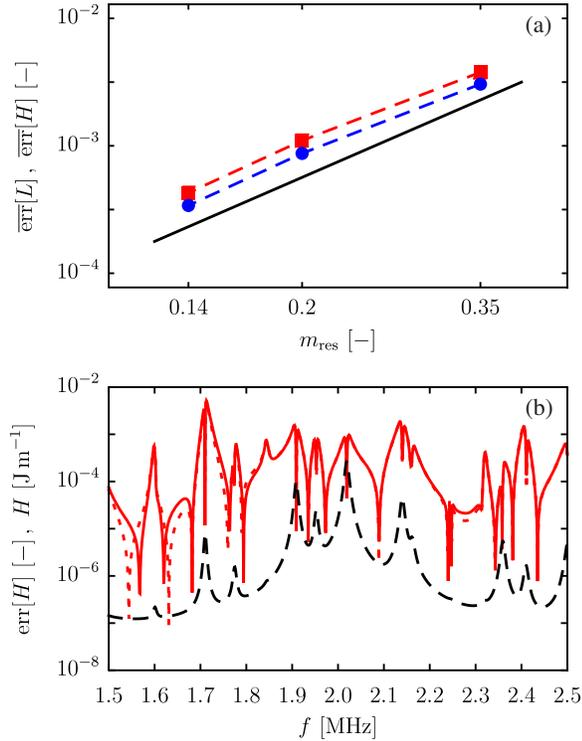
FIG. 4. (a) Log-log plot of  $\overline{\text{err}}[L(m_{\text{res}})]$  (filled circle) and  $\overline{\text{err}}[H(m_{\text{res}})]$  (filled square). The straight line is a reference slope corresponding to  $m_{\text{res}}^2$ . (b) Plot of the relative error for the real part (solid red line) and the imaginary part (dashed red line) of the Hamiltonian (dashed black line) for  $m_{\text{res}} = 0.14$ .
