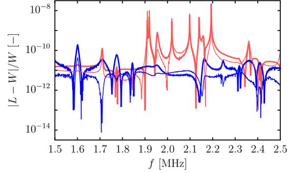
FIG. 5. Relative deviations for the real part (the light red lines) and imaginary part (the blue lines) of the Lagrangian  $\hat{L}$  from the external work  $\hat{W}$  versus frequency  $f$  for  $d_{\text{pz}} = 0 \mu\text{m}$ ,  $h_{\text{gl}} = 1100 \mu\text{m}$  for two mesh resolutions:  $m_{\text{res}} = 0.10$  (the thin lines) and  $m_{\text{res}} = 0.14$  (the thick lines).
