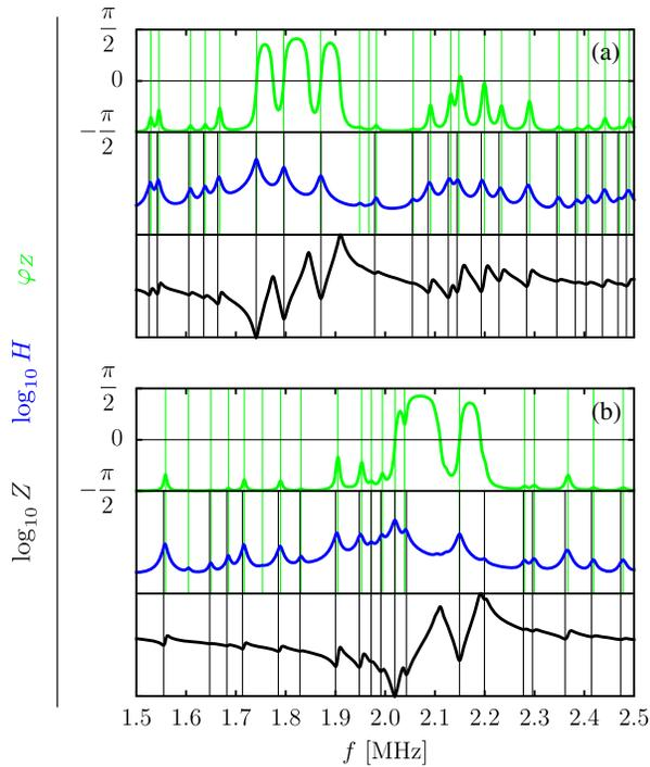
FIG. 10. Phase  $\varphi_Z$  (green lines), impedance  $Z$  (black lines), and energy  $H$  (blue lines) as function of the frequency  $f$  for Pyrex-silicon devices with  $d_{pz} = 250 \mu\text{m}$  for (a)  $h_{gl} = 200 \mu\text{m}$  and (b)  $h_{gl} = 1100 \mu\text{m}$ . Vertical black and green lines mark the frequencies obtained via the criterion equations (29)(i) and (29)(ii), respectively.
