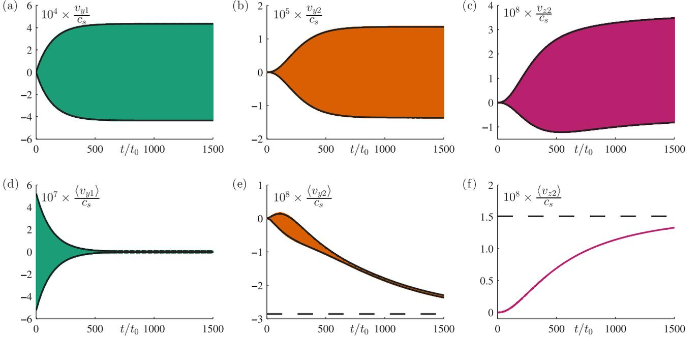
FIG. 6. (Color online) The velocity probes from Fig. 5, but now extended to the long time interval  $0 < t < 1500 t_0$ , showing the convergence towards a periodic state. The dashed lines in (e) and (f) indicate the magnitude of the steady time-averaged second-order velocity from the frequency-domain simulation Eqs. (11) and (12).
