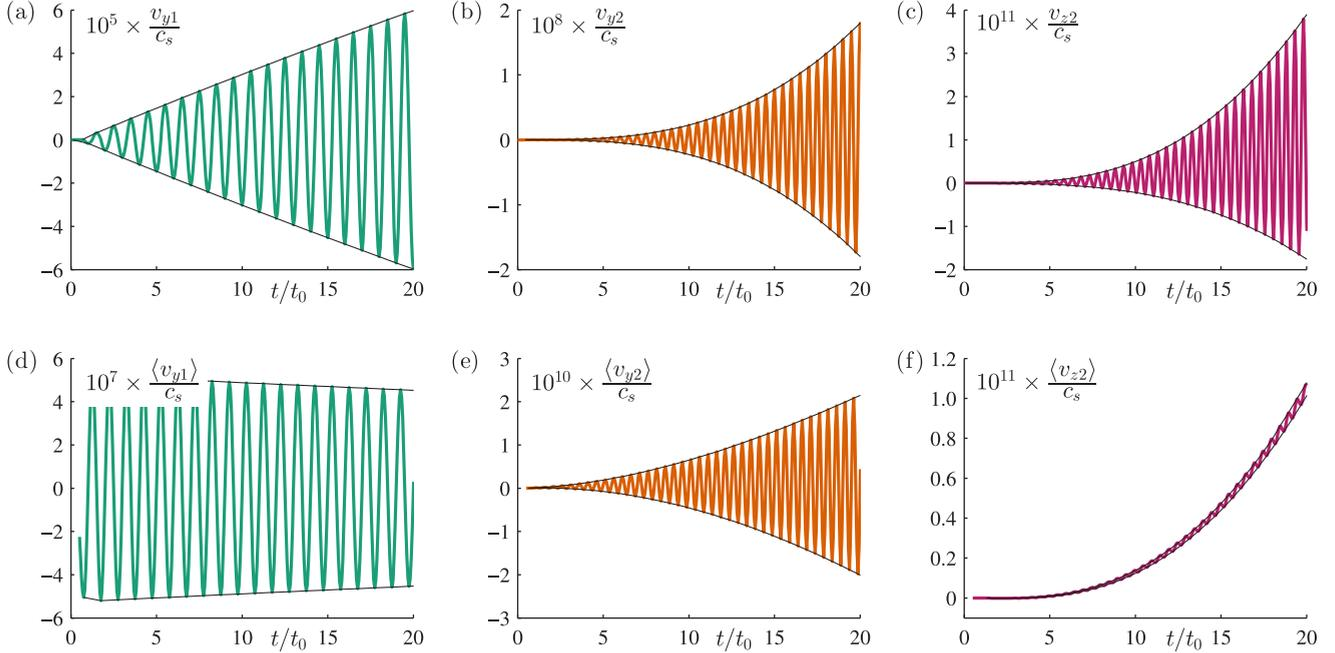
FIG. 5. (Color online) Velocity probes for the initial time interval  $0 < t < 20t_0$ . (a)–(c) Probes for the first- and second-order velocity (a)  $v_{y1}(0,0)$ , (b)  $v_{y2}(w/4,0)$ , and (c)  $v_{z2}(0,h/4)$ . (d)–(f) Running time-average Eq. (30) on an interval one oscillation period wide of the velocity probes in (a)–(c). The thick lines show the oscillating velocity probes while the thin lines emphasize the envelopes of the oscillations.
