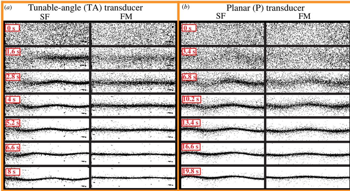
**Figure 6.** Dynamics of acoustophoresis patterns during (a): the first 8 s when actuating the device with the TA transducer and (b): the first 20 s when actuating the device with the planar (P) transducer. Both transducers were operated at  $U_{pp} = 20$  V at single frequency (SF, left panel) and frequency modulation (FM, right panel). The angle of the passive TA transducer is fixed at  $15^\circ$ .
