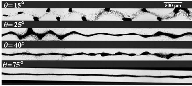
**Figure 4.** Steady-state acoustophoresis patterns of 5  $\mu\text{m}$  diameter particles after 10 min of SF actuation with the TA transducer for 4 different angles.
