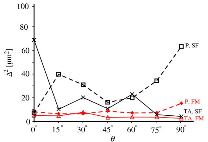
**Figure 3.** The variances  $\Delta^2$  from an ideal straight line of the patterns in figure 2 plotted as a function of the angle for planar (P) and TA transducer for both SF and FM actuation modes.
