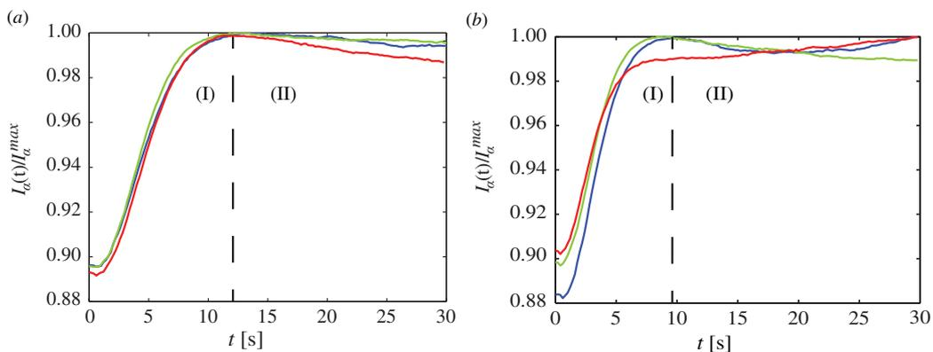
**Figure 9.** Reproducibility tests for the TA transducer,  $\theta = 15^\circ$ . Normalized light-intensity curves  $I_\alpha(t)/I_\alpha^{\text{max}}$  for (a) SF actuation, and (b) for FM actuation. Each experiment was repeated three times.
