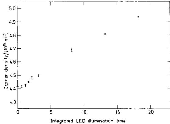
**Figure 4:** Carrier density in the high mobility channel from SdH-analysis of  $V_D$ . The illumination is by a red, 635 nm, LED
