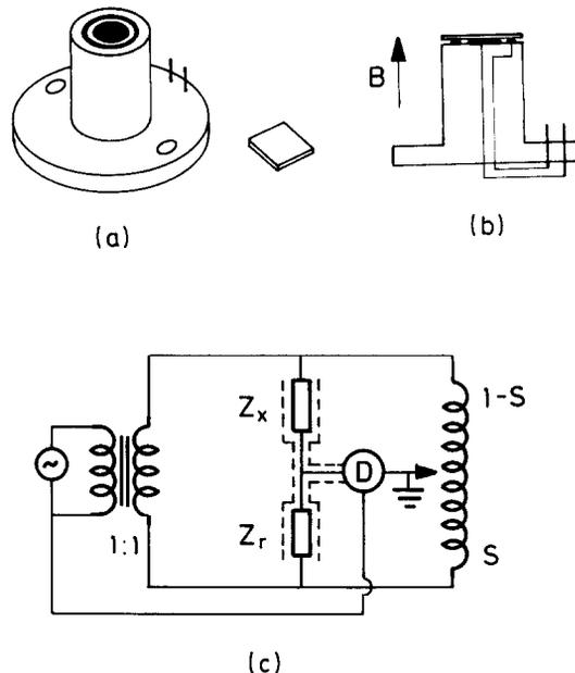
Figure 1: (a) The Corbino electrodes and the sample. (b) The mounted sample and the direction of the magnetic field. (c) The ac-bridge.
