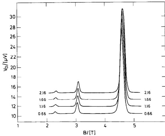
**Figure 3:** Bridge imbalance,  $V_D$ , versus magnetic field  $B$  at 4.2 K and 20 kHz. The numbers at the curves are integrated illumination times.
