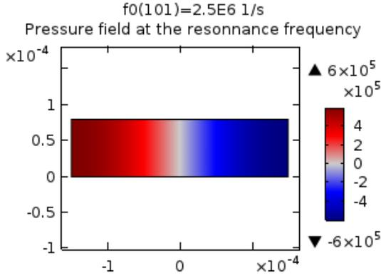
Figure 10: Pressure field(max:600kPa)
