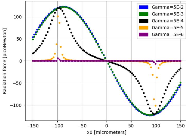
Figure 17: Radiation force on the infinitely hard and infinitely heavy particle for different values of the damping factor
