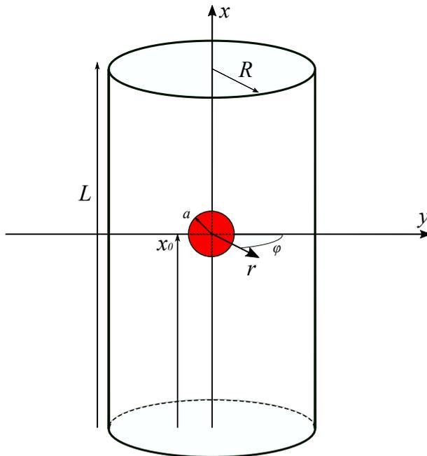
Figure 5: The studied microdevice: a cylindrical vertical structure of length  $L$  and radius  $R$  with a microparticle of radius  $a$  (red sphere) located on the axis at position  $x_0$
