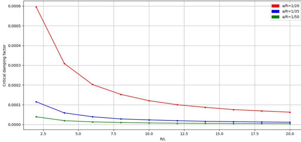
Figure 14: Critical damping factor  $\Gamma_c$  as function of the geometry of the device  $L$  and  $R$  as well as of the geometry of the particle  $a$
