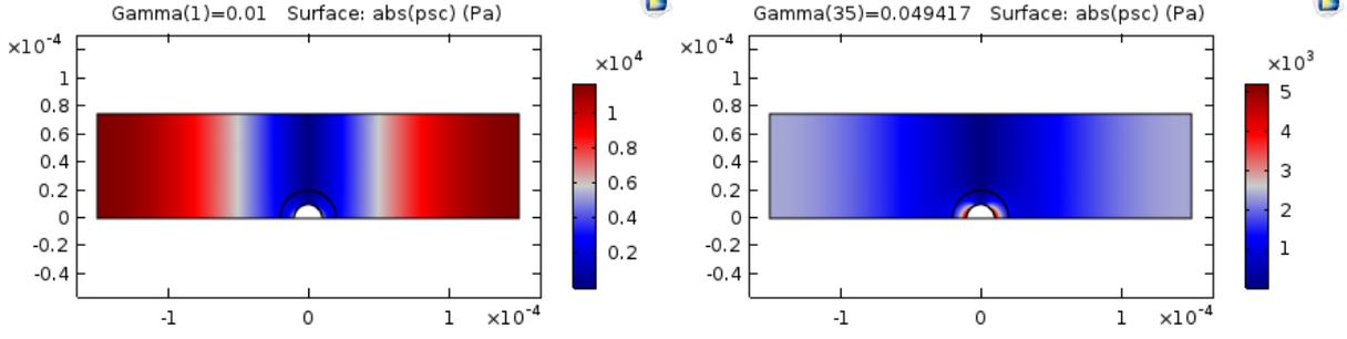
Figure 13: On the left, the absolute value of the scattered pressure field (max:  $10kPa$  for  $\Gamma = 0.01$  with  $L = 300\mu m$  and  $R = 75\mu m$  and on the right, the absolute value of the scattered pressure field (max:  $5kPa$  for  $\Gamma = 0.05$  with  $L = 300\mu m$  and  $R = 75\mu m$ )
