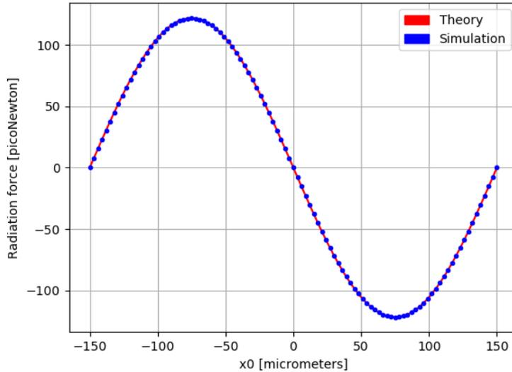
Figure 16: Comparison between the radiation force calculated with the formula issued of the scattering theory and the one obtained by the simulation with PML
