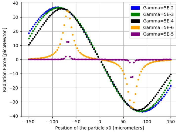
Figure 18: Radiation force on a droplet of glycerol for different values of the damping factor
