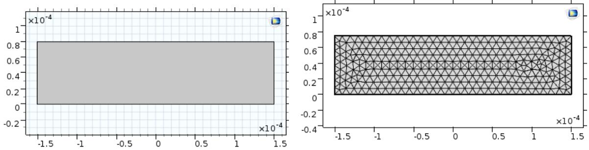
Figure 8: Geometry:  $L = 300\mu m$  and  $R = 75\mu m$
