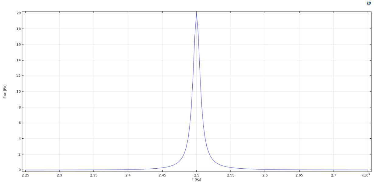
Figure 9: Acoustic energy density in function of the vibration frequency
