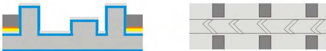
Figure 7.15: Permalloy is electroplated onto the electrically conducting structures.
