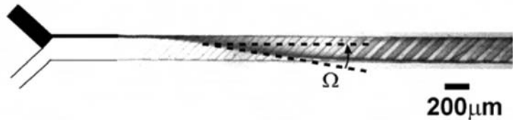
Figure 2.16: Predicted and measured values of the angle of the velocity below the top surface ( \tan \Omega ) in a channel with square grooves on the floor. In all cases w = 200\mu\text{m} , hc is given in micrometers, and the grooves are oriented at an angle \pi/4 with respect to the principal axis of the channel. Also shown is a micrograph taken from above of a stream of black dye flowing in a microchannel with pr = 140 \mu\text{m} , hc = 106 \mu\text{m} , and rc = 0.51 . The drawing on the left shows schematically the Y junction at the entrance of the channel; a narrow stream of black dye in water is injected alongside a broad stream of clear water (flow rate of the clear stream 20 times that of the dyed one). The average flow speed in the channel is 1 \text{ cm/s} (Reynolds number \sim 1 ) [46].
