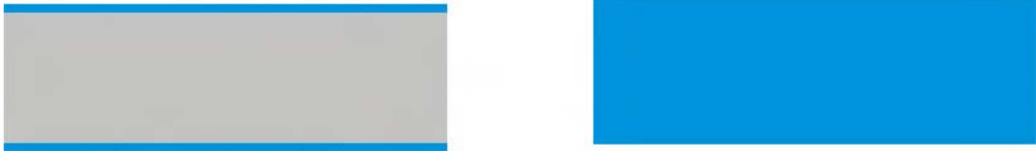
Figure 7.3: 1.2 \mu\text{m} of thermal oxide is grown. This is done in a wet atmosphere at 1100^\circ\text{C} .
