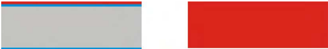
Figure 7.4: A 1.5 \mu\text{m} AZ5214 positive resist is applied. This is then exposed and developed (mask1) followed by a hardbake.
