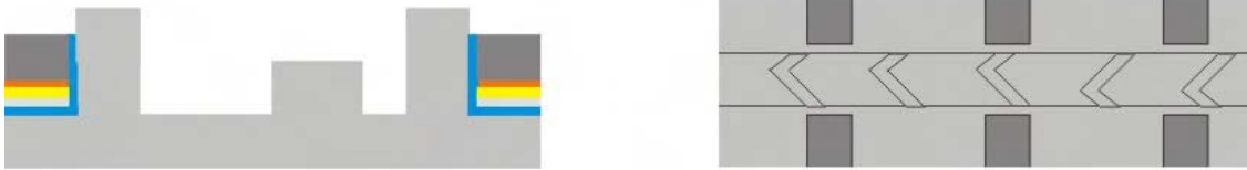
Figure 7.18: \text{SiO}_2 is etched from the wafer in BHF. This should also leave clean Si on the wafer.
