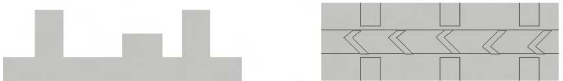
Figure 7.9: Elements and channels are etched, and the oxide is stripped in BHF.
