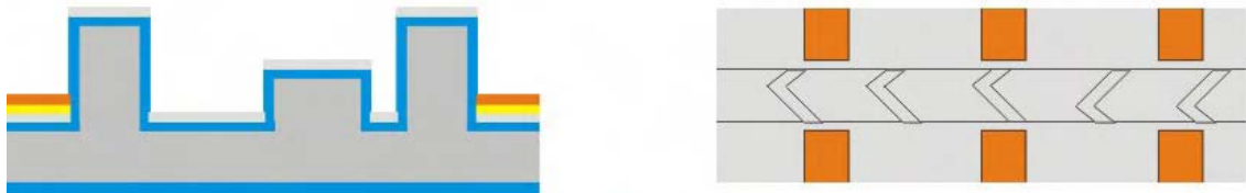
Figure 7.14: Au is etched away everywhere except where it is protected by Cu. If desired this can be followed by an etch of Cu.
