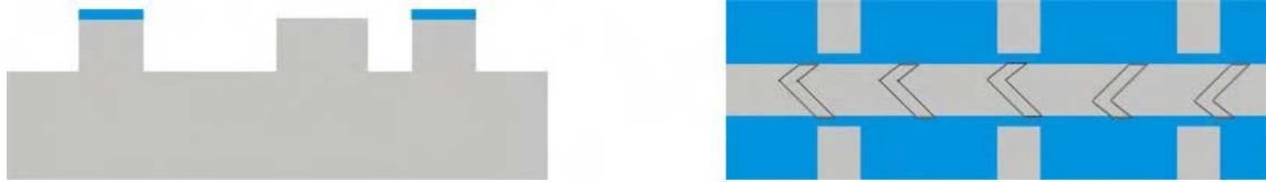
Figure 7.8: Elements, channels, and grooves are etched and the resist is stripped.
