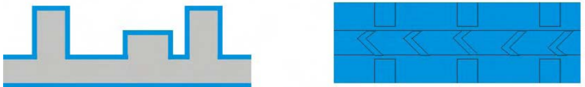
Figure 7.10: An RCA-clean is performed and then 0.1 \mu\text{m} thermal oxide is grown (wet at 1000^\circ\text{C} ).
