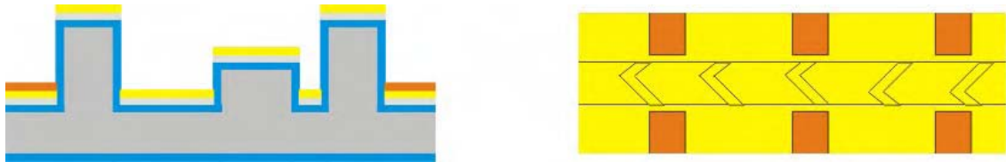
Figure 7.13: A short etch of Au is performed, followed by electroplating of 2.5 - 4 \mu\text{m} Cu.
