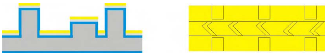
Figure 7.11: A seed layer of 5 nm Ti and 200 nm Au is deposited by e-beam evaporation.
