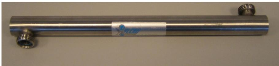
Figure 4.3: *The steel housing, in which the SiC-components were mounted. Either none, or just one permeate exit was used in each experiment.*
