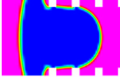
Figure 9.16: A wetting bubble nearly totally within the rough area. Dimensions: d = 300 \mu\text{m} , l = 60 \mu\text{m} , l_R = h_R = 30 \mu\text{m} , l_{O,R} = 0 \mu\text{m} .
