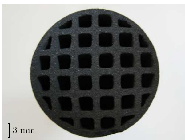
Figure 3.6: Picture of the cross-section of a 24-channel tube. The channels have a width of 3 mm and the walls have a thickness of 1 mm. The outer diameter of the tube is 25 mm.
