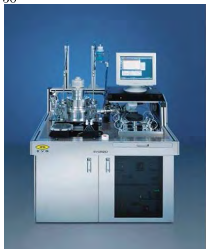
(a) The EVG-NIL bonder which was used to facilitate the SU-8 bonding. Source: : http://www.j-ml.com/images/eq/evg520he.jpg
