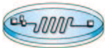
Figure 1.1: A schematic of a mixing channel. The devices consist of two layers: the substrate, in which the channels have been etched (blue), and the lid (transparent). The lid is attached to the substrate using a process called bonding. Holes have been drilled in the lid for access to the channels.
