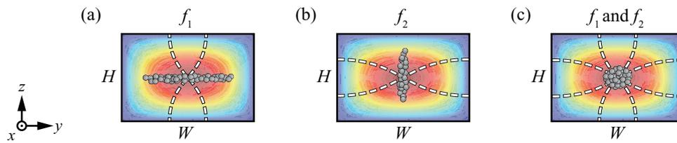
**Figure 1.** Schematic cross-section of a water-filled rectangular channel showing the working principle of 1D and 2D acoustophoresis, as microparticles experience the half-wave frequencies (a)  $f_1$  (1D vertical acoustophoresis), (b)  $f_2$  (1D horizontal acoustophoresis), and (c)  $f_1$  and  $f_2$  combined (2D acoustophoresis). The color plot represents the Poiseuille flow velocity profile from zero velocity (blue) to maximum velocity (red).
