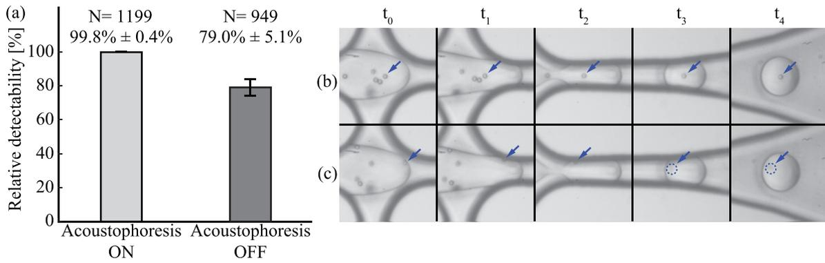
**Figure 4.** (a) Relative particle detectability with and without 2D acoustic actuation of the microparticles in the inlet channel. (b) and (c) zoomed still frames from the high-speed video showing encapsulation of a microparticle when the 2D acoustophoresis is (b) on and (c) off. The encapsulated microparticle in (b) can easily be detected optically whereas the encapsulated microparticle in (c) is out of focus.
