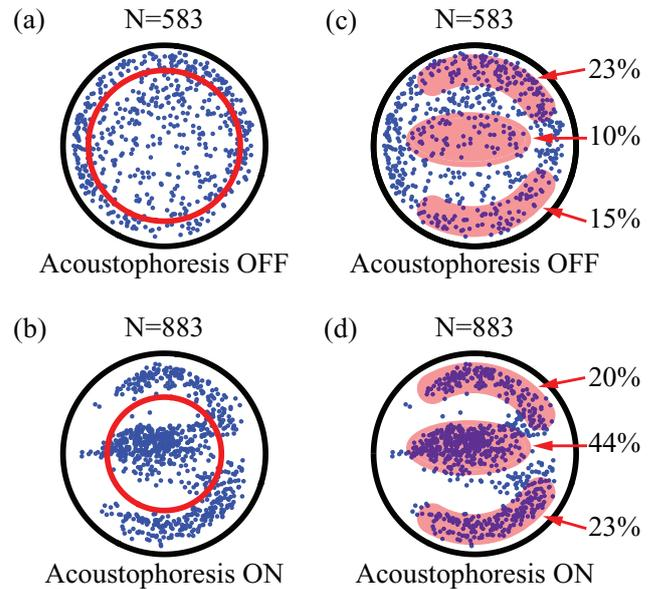
**Figure 5.** The positions (blue dots) of a total of 1466 single encapsulated microparticles are superimposed within a single droplet moving to the right. (a) and (b) the red circle indicates the median particle distance from the droplet center. (c) and (d) three regions with high particle concentration are marked.
