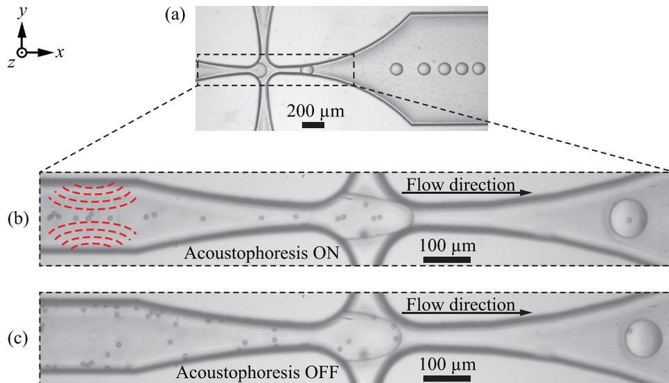
**Figure 3.** (a) Photograph showing the droplet formation process. Inserts are zoomed still frames from the high-speed video showing how the microparticles are aligned during the droplet formation processes when the 2D acoustophoresis is (b) on, and (c) off.
