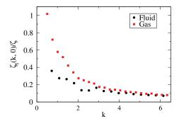
FIG. 6. Zero frequency longitudinal spin viscosity as a function of wavevector relative to  $\zeta$  given in Table I. The kernel for the liquid state point is zero for all wave vectors shown here. As in Fig. 5 the data were averaged and a Hann window<sup>36</sup> was applied before Fourier-Laplace transforming.
