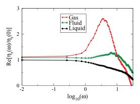
FIG. 5. Real part of the rotational viscosity for the three different state points for  $\omega > 0.01$  and relative to the zero frequency value,  $\eta_r(0)$ , given in Table I column three. Before performing the Fourier-Laplace transform all data were averaged and a Hann window<sup>36</sup> was applied to the resulting single data set in order to obtain the best possible curves.
