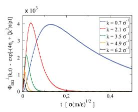
FIG. 1. Liquid chlorine. Comparison between Eq. (13b) and the approximation given by Eq. (28b) for different wavevectors. The units are reduced molecular dynamics units,  $\sigma=3.3321$  Å,  $\epsilon=2.46210\times10^{-21}$  J and m=35.45 g/mol.
