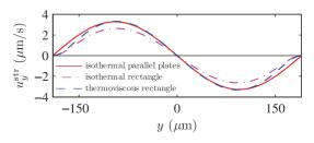
FIG. 4. (Color online) Numerical simulation of the horizontal component  $u_y^{\text{str}}$  of the streaming velocity in the ultrasound symmetry plane at z = 0. In this plane the vertical component is zero  $u_z^{\text{str}} = 0$ . Three cases are shown: the isothermal parallel-plate channel [Eq. (7)], the isothermal rectangular channel [Eq. (8)], and the thermoviscous rectangular channel [Eq. (10)].
