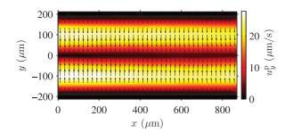
FIG. 6. (Color online) Experimental micro-PIV measurement of acoustophoresis in the horizontal ultrasound symmetry plane of 1- $\mu$ m-diam polystyrene particles suspended in water and driven at the piezo frequency f = 1.940 MHz corresponding to  $\lambda/2 = w$ , temperature 25 °C, and voltage  $U_{pp}^* = 7.94$  V. The arrows represent the measured velocity vectors  $\boldsymbol{u}^p$  and the grayscale (colorscale) their magnitude  $u^p$  normalized to  $U_{pp}^*$  [see Eq. (20)].
