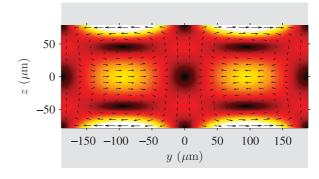
FIG. 3. (Color online) Vector plot (black arrows) of the acoustic streaming U and color plot of its magnitude U from zero (black) to maximum (white) given by Rayleigh's analytical expression [Eqs. (12)] and valid for a shallow isothermal liquid slab ( $\lambda \gg h$ ) between two parallel plates (gray) of distance h driven by a standing ultrasound pressure wave  $p_1 = p_a \cos[n\pi(y/w + 1/2)]$  for n = 1 and  $w = 377 \ \mu$ m.
