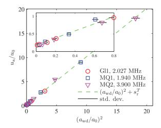
FIG. 9. (Color online) Plot of the measured normalized acoustophoretic particle velocity amplitude  $u_a/u_0$  versus the square  $(a_{\rm wd}/a_0)^2$  of the normalized wall-drag-corrected particle radius. The dashed line is a fit to Eqs. (12).
