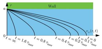
Fig. 3 The evolution in time from the initial Poiseuille paraboloid at t = 0 to a zero velocity profile at  $t = \infty$  of the velocity profile  $v_x(r, t)$  in a cylindrical channel of radius a for a decelerating Poiseuille flow due to the abrupt disappearance of the driving pressure  $\Delta p$  at t = 0. The time is expressed in units of the inertial time scale  $\tau_{\text{iner}} = a^2/(4v)$  of eqn (14). Adapted from ref. 3.
