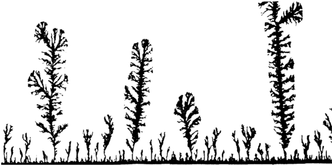
Figure 1.1: Photograph of zinc dendrites formed on a copper electrode. Adopted from Trigueros P. P. et al. , Pattern morphologies in zinc electrodeposition [10]
