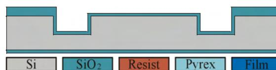
Figure 4.1: Cross sectional view of the silicon part of the device. The nanochannel is shown in the middle surrounded by inlet and outlet channels etched directly in the silicon. Notice the difference in thickness between the thick oxide on top defining the nanochannel height and the thin oxide layer in nano and inlet channels ensuring hydrophilic surfaces.
