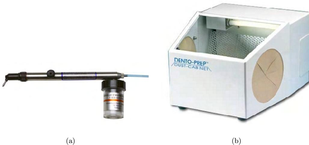
Figure 5.1: Equipment for powder blasting. (a) Microetcher. Pressurized air sucks up the blasting material from the reservoir and emits it at high speed through the nozzle. (b) Dust cabinet equipped with light and filtered extraction reduces the amount of dust leaked to the surroundings. Pictures from [19] and [20] respectively.
