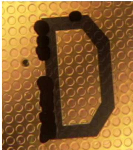
Figure 6.14: The letter D has been created by making a liftoff of the gold. It is evident that where the gold has been removed there is an increased risk of unwanted electroplating
