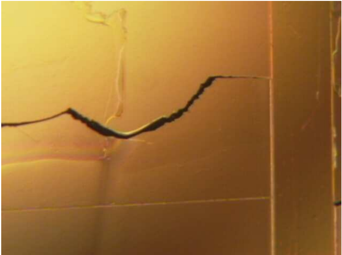
Figure 5.16: Side of square structure. Top right area: Both layers of SU-8 removed. Top left area: SU-8 2002 remains while SU-8 2050 has been removed. Bottom Area: Both layers of SU-8 remain. Notice how the vertical line separating the top areas continues below.
