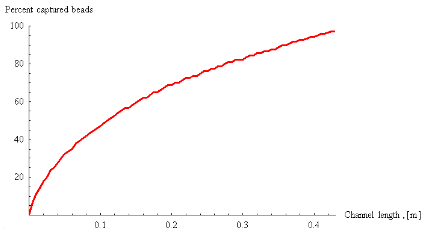
Figure 3.18: The percentage of captured beads as a function of the channel length for a single with a bar width of 50\mu\text{m} and a with bar spacing of 750\mu\text{m} found from the simulations.
